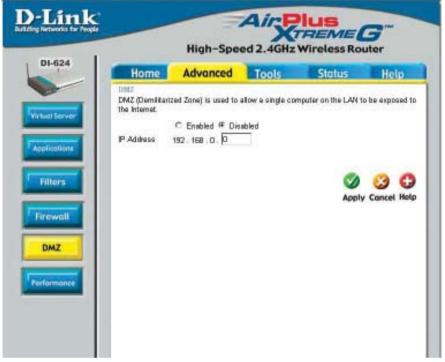
If you have a client PC that cannot run Internet applications properly from behind the DI-624, then you can set the client up for unrestricted Internet access. It allows a computer to be exposed to the Internet. This feature is useful for gaming purposes. Enter the IP address of the internal computer that will be the DMZ host. Adding a client to the DMZ (Demilitarized Zone) may expose your local network to a variety of security risks, so only use this option as a last resort.
