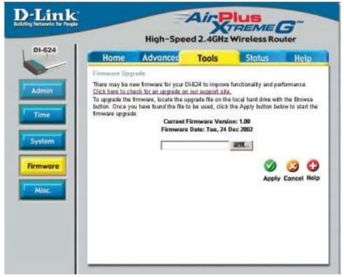
You can upgrade the firmware of the Router here. Make sure the firmware you want to use is on the local hard drive of the computer. Click on **Browse** to browse the local hard drive and locate the firmware to be used for the update. Please check the D-Link support site for firmware updates at http://support.dlink.com. You can download firmware up-grades to your hard drive from the D-Link support site.
